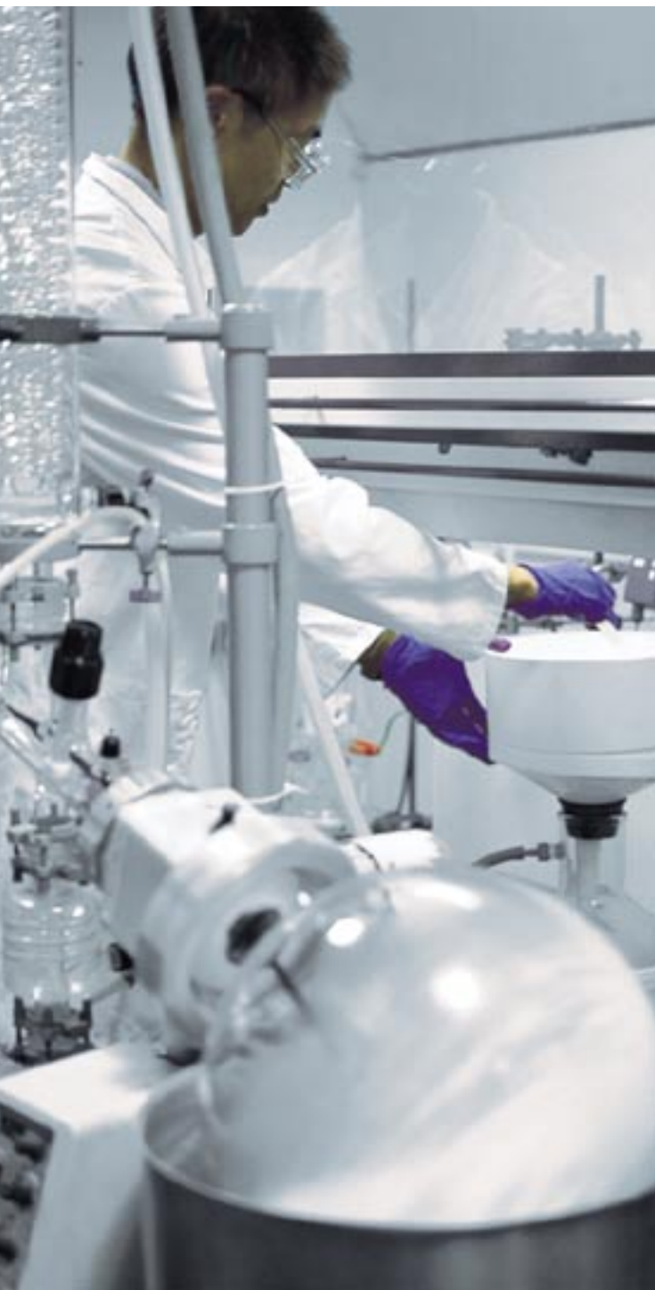
Filtration of a drug intermediate during a GMP custom preparation
